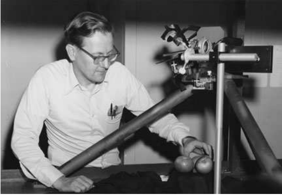
Fig. 8.4. Juris Upatnieks at ERIM, Ann Arbor, MI, 1979. The photograph shows the hologram recording setup, without the film holder, of a 12 in. diameter 360° hologram recorded for the Museum of Holography (MIT MoH collection).
