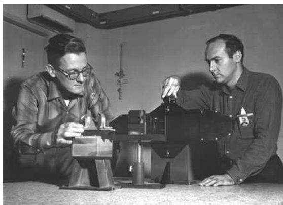
Fig. 4.11 Juris Upatnieks and Emmett Leith at optical table, December 1963. The apparatus, described in press reports as a hologram camera, was in fact a plate holder intended to allow multiple exposures and was probably never used. The actual apparatus was distributed over a large solid table. 102 (University of Michigan News Service, Leith collection).
